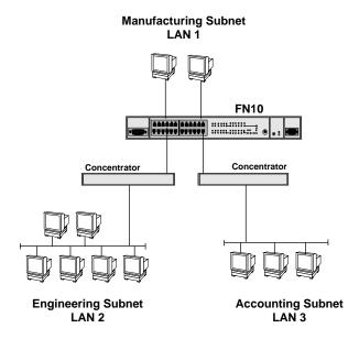
Figure 5-1 Using Filters to Restrict Access to an Adjoining Network Segment
